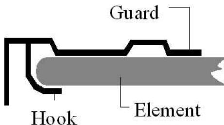
After cleaning the oven, ensure that the oven element is securely clipped into the hook of the element guard. Failure to observe this precaution will allow the element to rest on and damage the oven enamel.
